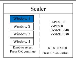
**Step 5:** Click "MENU" to return to the main menu interface, enter Menu - More - Common Functions - Partial Display, enter the part display setting interface, and set the size and position of the partial interception of each signal source.
